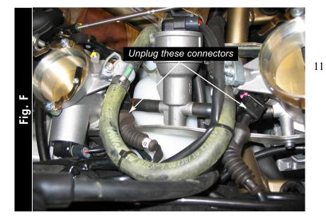
Unplug the stock connectors from the injectors (Fig F). Release the spring clips to remove each connector.
