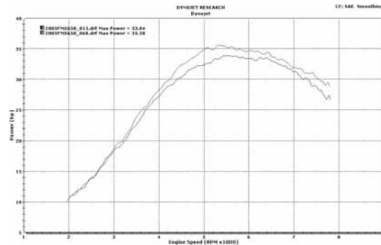
This graph shows a typical gain with a Dynojet jet kit.
