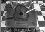
Fig. B Remove this snorkel from the airbox
