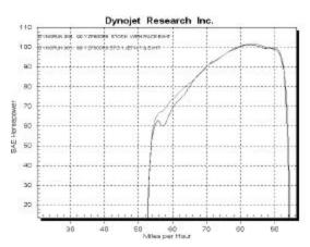
This graph shows a typical gain with a Dynojet jet kit.
