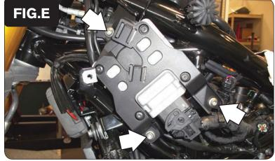
11 Loosen the bike's ECM by removing the three bolts shown in Figure E.
