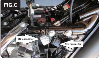
Route the stock ECM connectors that were disconnected in step 2 under the frame tube as in Figure C.
