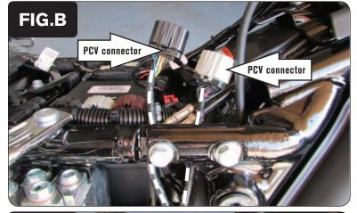
Route the Female connectors of the PCV behind the frame tube on the right side of the bike as in Figure B. Slide the harness towards the rear of the bike.
