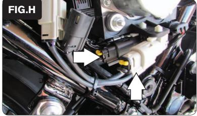
9 Plug the Dynojet O2 Optimizers into the stock wiring harness (Fig. H).
