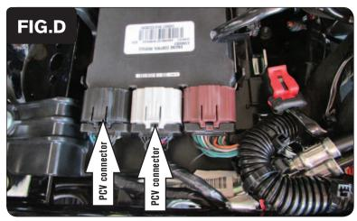
5 Plug the PCV connectors into the stock ECM (Fig. D).
