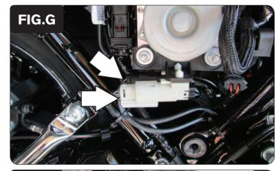
8 Locate the stock O2 sensor connections and unplug both connectors (Fig. G).
