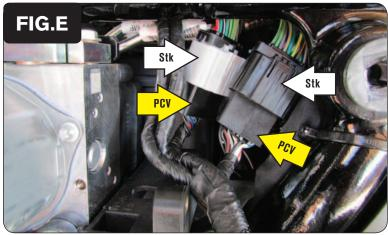
Plug the Male connectors of the PCV into the stock Female connectors (Fig. E).
