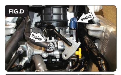
7 Unplug the Fuel Injector. Unplug the Throttle Position Sensor (Fig. D).
