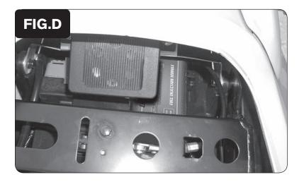
6 With the supplied velcro, attach the PCV module towards the rear most area of the inner fender (Fig. D). Use the supplied alcohol swab to clean both surfaces before attaching.
