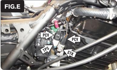
10 Plug the connectors from the PCV wiring harness in-line of the TPS and the stock wiring harness (Fig. E).
