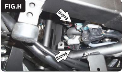
At the top of the engine, unplug the stock wiring harness from both of the Ignition Coils (Fig. H).
