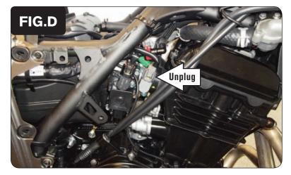
9 Locate and unplug the primary Throttle Position Sensor on the right hand side of the throttle bodies (Fig. D).
