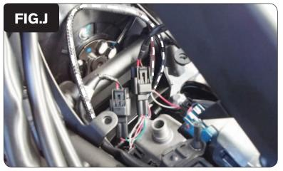
Plug the PCV wiring harness in-line of the stock wiring harness and the Ignition Coils (Fig. J).
