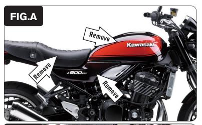
1 Remove the seat, the right and left side body panels and the fuel tank (Fig. A).
