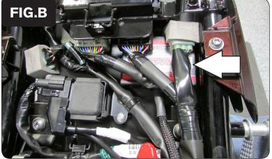
Install the PCV in the tail section near the ECU (Fig. B).
