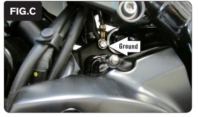
4 Secure the PCV ground wire with the small ring lug to the common ground location on the left side of the engine (Fig. C).
