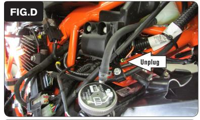
8 Unplug the stock wiring harness from the ignition coil (Fig. D).
