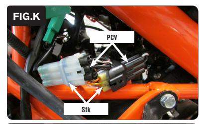
16 Plug the PCV in-line of the stock CPS and wiring harness (Fig. K).
