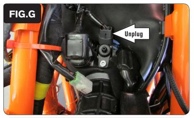
12 Unplug the wiring harness from the fuel injector (Fig. G).
