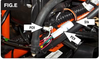
9 Plug the PCV in-line of the stock wiring harness and stock ignition coil (Fig. E)
