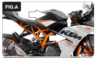
1 Remove the battery access cover, fuel tank cover, and side panels (Fig. A).
