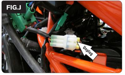
Unplug the stock crank position sensor connector (Fig. J).This is a WHITE, 6 pin connector near the FRT, LH side of the cylinder head.
