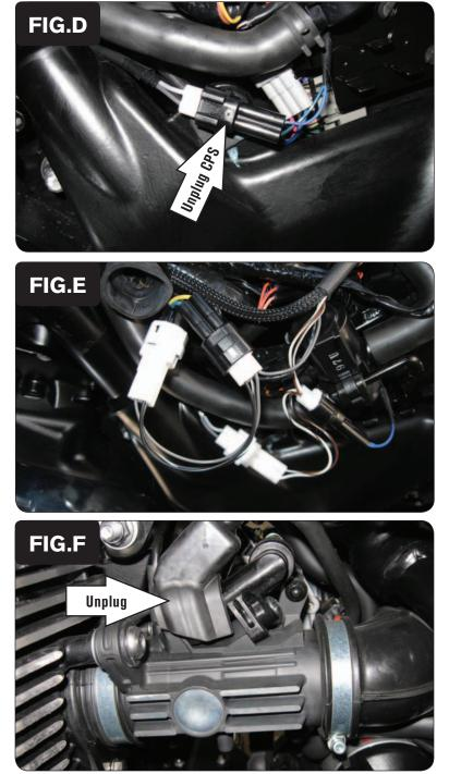
7 Locate the Crank Position Sensor connectors under the left hand side cover. Unplug this connector pair (Fig. C).
