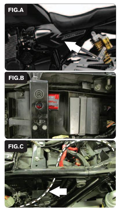
Remove the seat and left side panel (Fig. A).
