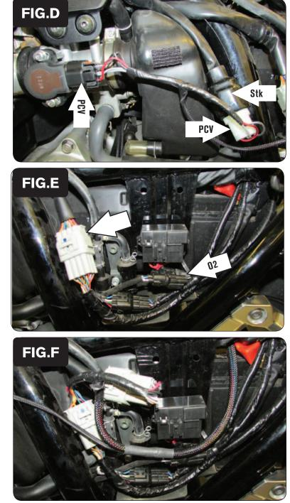
4 Plug the PCV in-line of the stock Throttle Position Sensor and wiring harness (Fig. D).
