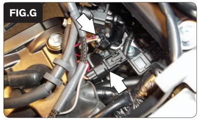
Plug the PCV wiring harness in-line of the Fuel Injector and the stock wiring harness (Fig. G).
