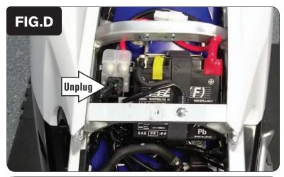
5 Unplug the stock wiring harness from the bike's starter solenoid just right of the battery (Fig. D).
