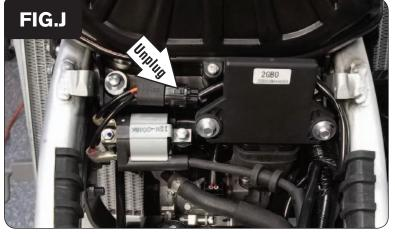
Unplug the stock wiring harness from the Ignition Coil sub-connector (Fig. J).
