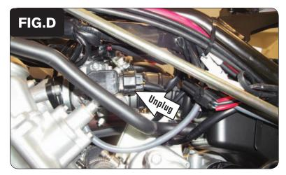
7 Unplug the Throttle Position Sensor from the left side of the throttle body (Fig. D).
