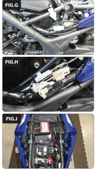
9 Unplug the crank position sensor connector (Fig. G).This is a BLACK connector pair on the left side of the motorcycle.
