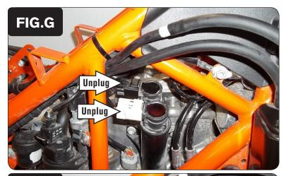
13 On the right side of the engine, locate and unplug the stock BLACK 2-pin connector from the inner coil stick and the stock WHITE 2-pin connector from the outer coil stick (Fig. G).
