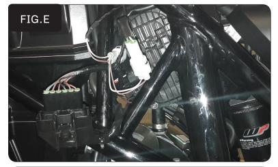
Plug the PCV in-line of the stock TPS and wiring harness (Fig. E). 9
