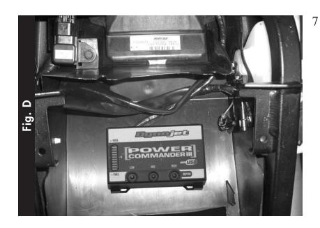
Install the Power Commander in the tail section. Make sure to use the supplied alcohol swab to clean the inner rear fender before attaching the Power Commander. Use the supplied velcro to secure the unit to the inner rear fender (Fig. D).
