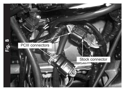
4 Plug the connectors from the Power Commander in-line of the stock connector (Fig. B).
