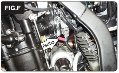
8 Use the supplied Positap to attach the unterminated GREY wire of the PCFC wiring harness to the stock LIGHT BLUE wire of the Throttle Position Sensor connector on the stock wiring harness (Fig. F).
