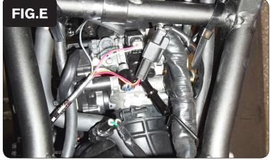
Plug the pair of 2-pin PCFC connectors in-line with the Fuel Injector and the stock wiring harness (Fig. E).
