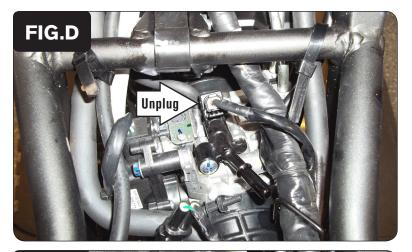
6 Locate and unplug the Fuel Injector at the top of the throttle body (Fig. D).
