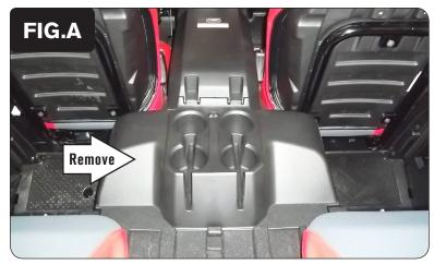
1 Remove the center console panel in the rear passenger area to access the engine compartment (Fig. A).
