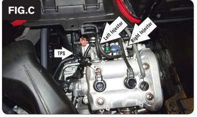
Unplug both Fuel Injectors and the Throttle Position Sensor from the throttle bodies (Fig. C).
