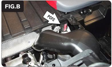
2 Use the supplied Velcro to secure the PCFC module in the engine compartment at the locations shown in Figure B.
