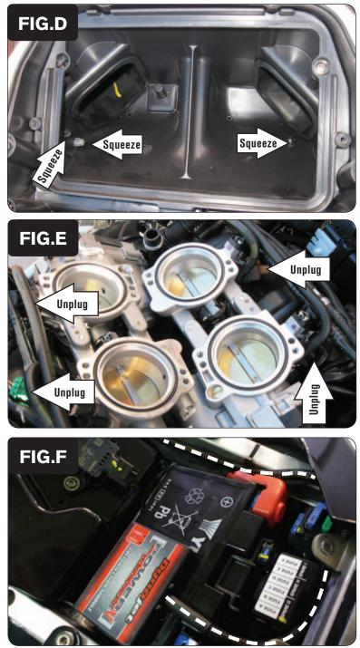
7 Remove the lower half of the airbox. There are 3 pins that must be squeezed to be removed (Fig. D).
