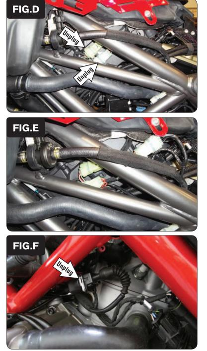
Beneath the rear of the fuel tank on the left side of the bike, locate and unplug the stock Fuel Injector connector and the stock Throttle Body Servo connector for the Vertical cylinder.
