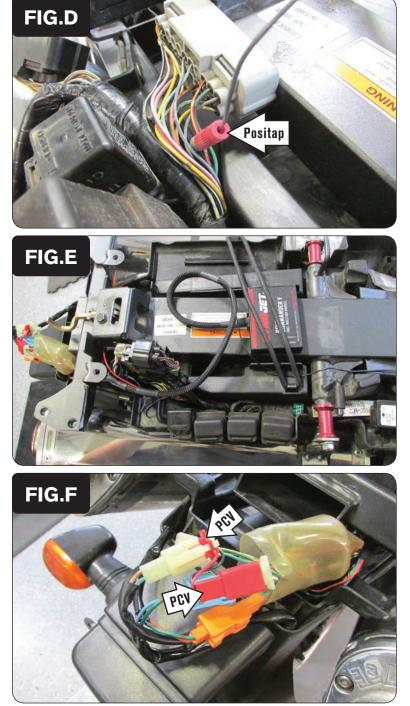
Use one of the supplied Positaps to attach the PCV GREY wire to the stock RED/YELLOW wire (pin #9) of the stock GREY ECM connector (Fig. D).
