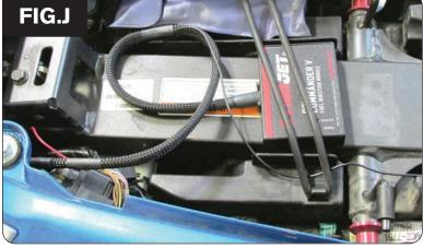
10 Route the PCV ground wire to the bike's battery (Fig. G).
