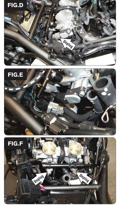
7 Unplug the Throttle Position Sensor at the right side of the throttle bodies (Fig. D).
