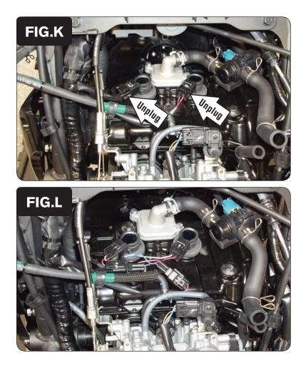
13 Unplug the stock wiring harness from both Ignition Coil sticks (Fig. K).
