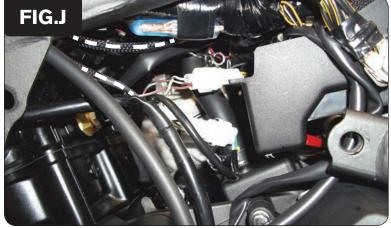
10 Plug the PCV wiring harness in-line of both Fuel Injectors and the stock wiring harness (Fig. G).
