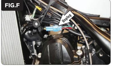
12 Unplug the stock Crank Position Sensor connectors (Fig. F).
