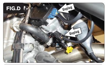
9 Unplug the Fuel Injector and the Throttle Position Sensor.
