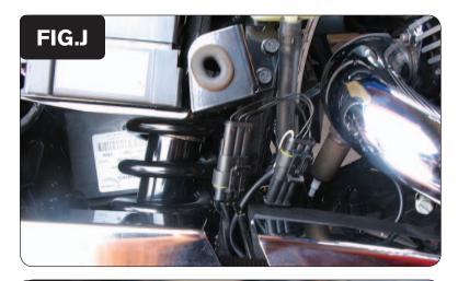
17 Plug the PCV harness in-line of the stock wiring harness and crank pickup coil connector (Fig. J).
