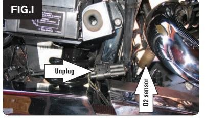
Locate the crank pickup coil connector on the right hand side of the bike near the rear shock (Fig. I).
