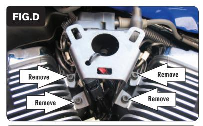
9 Remove the 4 bolts that hold the Ignition coil bracket to the engine (Fig. D).
