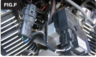
Plug the PCV wiring harness in-line of the stock wiring harness and Ignition coil (Fig. F).
