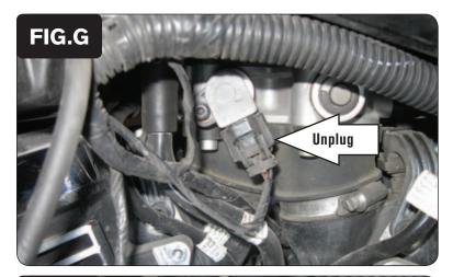
Locate the Throttle Position Sensor wiring harness on the left hand side of the throttle bodies. Unplug the stock wiring harness from the TPS (Fig. G).
