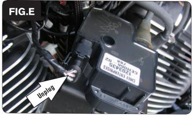
10 Unplug the stock wiring harness from the Ignition Coil (Fig. E).
