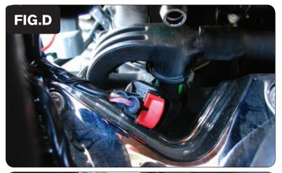
6 Locate the stock wiring harness at the rear injector (Fig. D). Lift up on the RED clip and unplug the injector connector.
