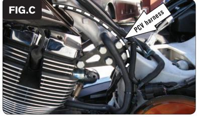
Route the PCV harness along the backbone of the frame along the left side of the bike and go towards the throttle body (Fig. C).
