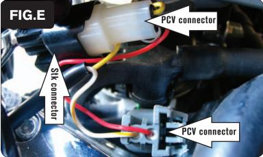
7 Plug the pair of leads with the YELLOW colored wires from the PCV in-line of the stock wiring harness and fuel injector (Fig. E)
