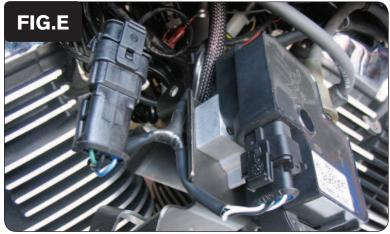
Plug the PCV wiring harness in-line of the stock wiring harness and Ignition Coil (Fig. E).
