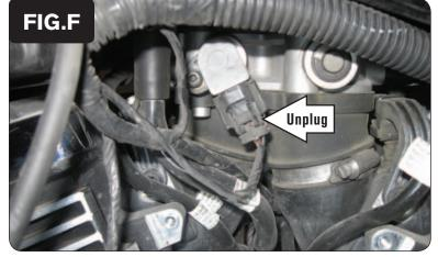
Locate the Throttle Position Sensor wiring harness on the left hand side of the throttle bodies. Unplug the stock wiring harness from the TPS (Fig. G).
