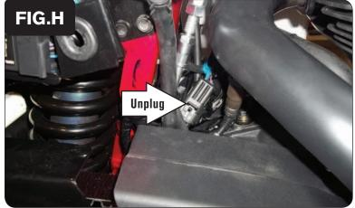
Locate the Crank Position Sensor connectors on the right hand side of the bike near the rear shock (Fig. H).
