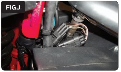
18 Plug the PCV harness in-line of the stock wiring harness and crank pickup coil connector (Fig. J).
