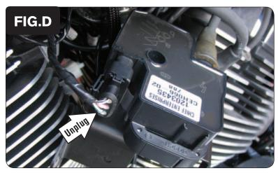
11 Unplug the stock wiring harness from the Ignition Coil (Fig. D).
