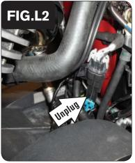
21 Unplug the front and rear stock O2 sensor connectors (Fig. L1 & L2).
