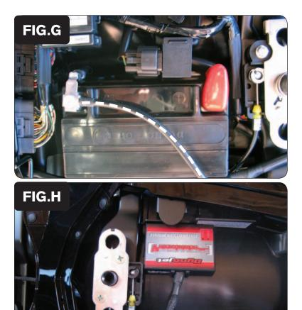
9 Secure the ground wire of the PCV wiring harness with the small ring lug to the negative (-) terminal of the bike's battery (Fig. G).
