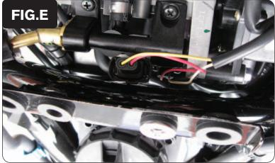
Plug the YELLOW colored wires of the PCV in-line of the stock wiring harness and rear injector (Fig. E).
