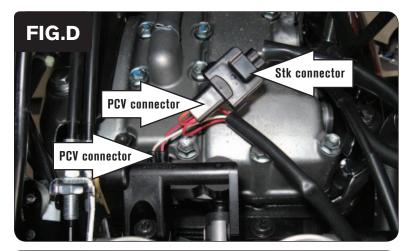
7 Plug the ORANGE colored wires of the PCV in-line of the stock wiring harness and front injector (Fig. D).
