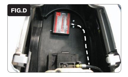
7 Using the supplied Velcro, secure the PCV module in the tail section (Fig. D).
