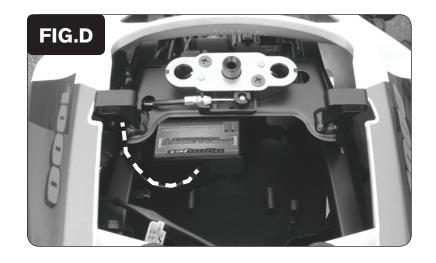
Using the supplied Velcro, secure the PCV module in the tail section (Fig. D).
