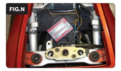
19 Using the supplied Velcro, secure the PCV module in the tail section (Fig. N). Clean both surfaces with the supplied alcohol swab prior to applying the
