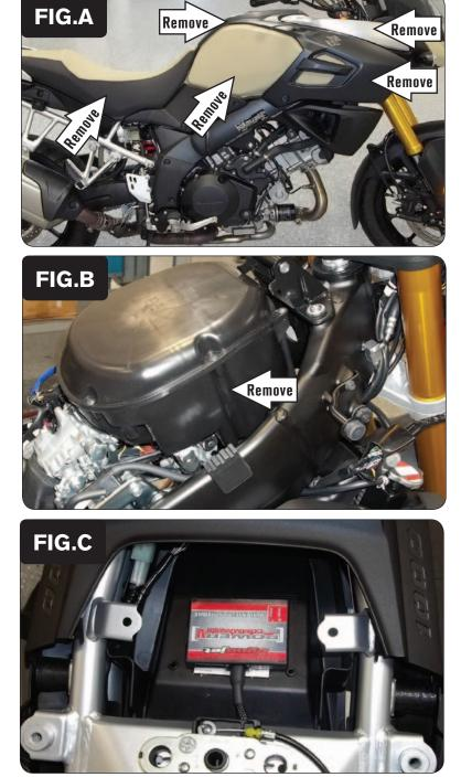
1 Remove the seat, the body panels surrounding the fuel tank, and remove the fuel tank (Fig. A).
