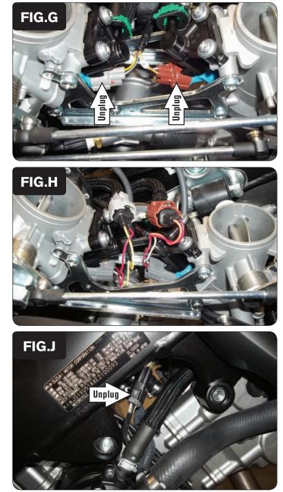
8 Locate and unplug the stock Fuel Injectors, which are located between the throttle bodies (Fig. G).
