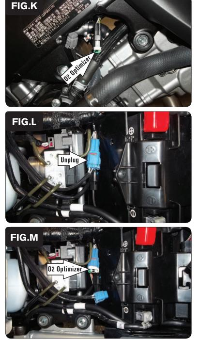
12 Plug one of the supplied O2 Optimizers into the bike's wiring harness in-place of the stock Front O2 Sensor (Fig. K).
