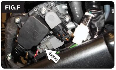
10 Unplug the lower primary Throttle Position Sensor connector with the GREY connector (Fig. F).
