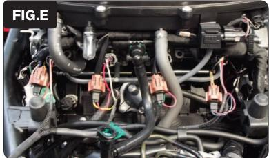
9 Plug the PCV wiring harness in-line of each fuel injector and the stock wiring harness (Fig. E).
