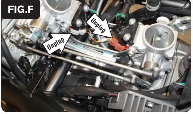
8 Locate and unplug both of the stock connector pairs for both of the bike's Ignition Coils (Fig. D).
