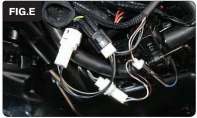
Plug the connectors from the PCV in-line of the stock Throttle Position Sensor connectors and the stock Crank Position Sensor connectors (Fig. E).
