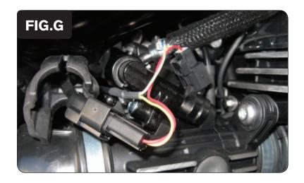
10 Plug the PCV connectors in-line of the stock wiring harness and fuel injector for both cylinders (Fig. G).
