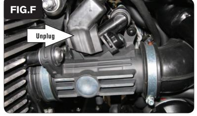
9 Unplug the stock wiring harness from both fuel injectors (Fig. F).
