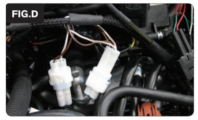
9 Plug the PCV harness in-line of the stock wiring harness and crank position sensor harness (Fig. D).
