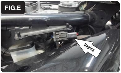
9 Locate and unplug the stock Crank Position Sensor connectors under the right frame rail under the seat (Fig. E).
