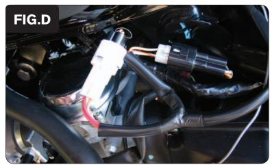
8 Plug the PCV wiring harness in-line of the stock connectors (Fig. D).
