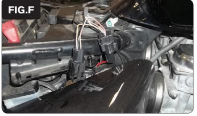
10 Plug the PCV in-line of the stock Crank Position Sensor connectors (Fig. F).
