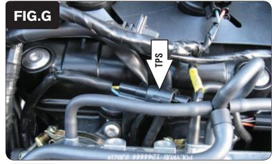
Locate and unplug the stock Throttle Position Sensor connectors (Fig. G).
