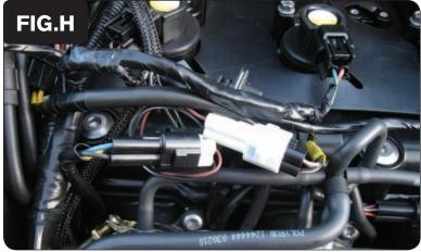
Plug the pair of WHITE 3-pin connectors from the PCV in-line of the stock TPS connectors (Fig. H).
