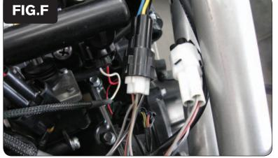
6 Plug the PCV harness in-line of the stock wiring harness and each fuel injector.
