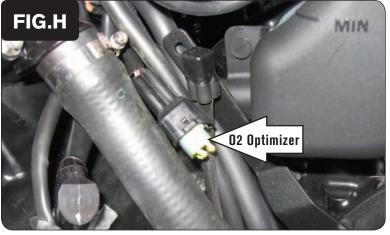
12 Plug the Dynojet O2 Optimizer into the stock wiring harness (Fig. H).
