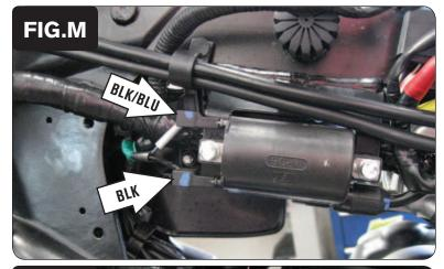
17 Unplug the stock wires from the Left Ignition Coil (Fig. M).
