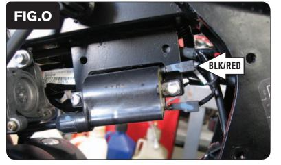
Unplug the stock BLACK/RED (signal) wire from the Right Ignition Coil (Fig. O).
