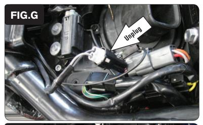
9 Unplug the stock 2-pin connectors (1 BLACK, 1 WHITE) under the seat for the bike's Crank Position Sensor (Fig. G).
