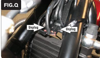
Locate and unplug the connectors for the bike's stock O2 sensors (Fig. Q).
