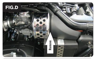
Remove the left side cover above the battery, starting with the chrome cover, then the plastic cover behind it (Fig. D).
