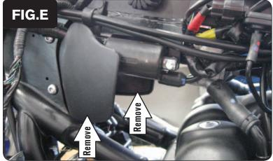
Remove the two covers at the front of the frame that cover both of the bike's Ignition Coils (Fig. E).
