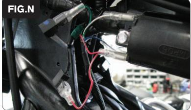
18 Plug the pair of PCV wiring harness leads with the RED colored wires in-line of the stock BLACK wire and the Left Ignition Coil (lower, BLACK tab).
