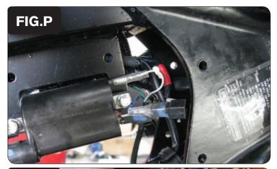
21 Plug the pair of PCV wiring harness leads with the BLUE colored wires in-line of the stock BLACK/RED wire and the Right Ignition Coil (upper, GREY tab).
