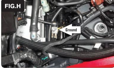
Secure the ground wire of the PCV wiring harness with the small ring lug to the stock ground location on top of the engine case (Fig. H).
