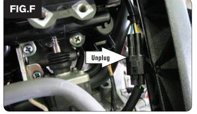
7 Locate and unplug the stock wiring harness from the bike's Crank Position Sensor (Fig. D).
