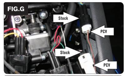
10 Plug the PCV harness in-line of the stock TPS connectors (Fig. G).
