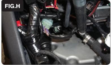
Plug the pair of 6-pin connectors of the PCV wiring harness in-line of the stock CPS connectors (Fig. H).
