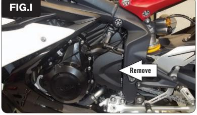
Remove the lever arm from the gear shift pivot shaft on the gearbox; and remove the counter shaft sprocket cover (Fig. I).
