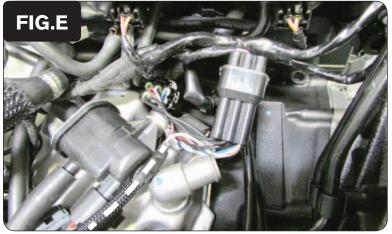
Plug the PCV wiring harness in-line of the stock Crank Position Sensor connectors (Fig. E).
