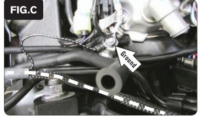
Secure the PCV ground wire with the small ring terminal to the stock common ground bolt at the top of the engine case (Fig. C).
