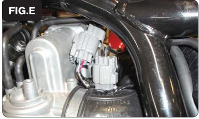
9 Plug the PCV wiring harness in-line of the TPS and the stock wiring harness (Fig. E).
