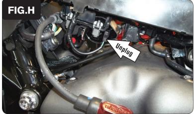
12 Unplug the GREEN/PINK signal wire from the right cylinder Ignition Coil (Fig. H).
