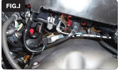
Plug the BLUE and WHITE/BLUE PCV wires in-line of the right cylinder Ignition Coil and the stock signal wire (Fig. J).
