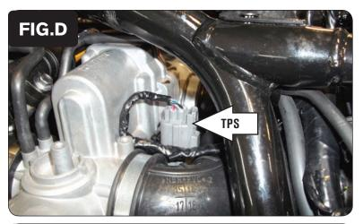
8 Unplug the stock Throttle Position Sensor connector located on the left side of the throttle bodies (Fig. D).
