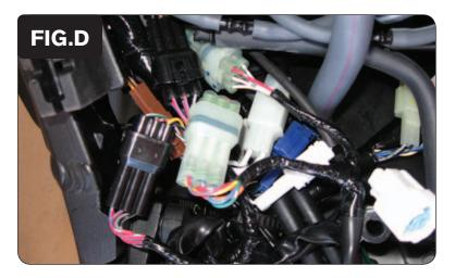
Plug the PCV connectors in-line of the throttle bodies and main wiring harness (Fig. D). Plug the colored connectors from the PCV into the matching stock connectors.
